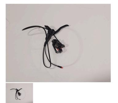
Gio Lightning Parts Front Brake Lever and Caliper (left) (Gio Lightning)
